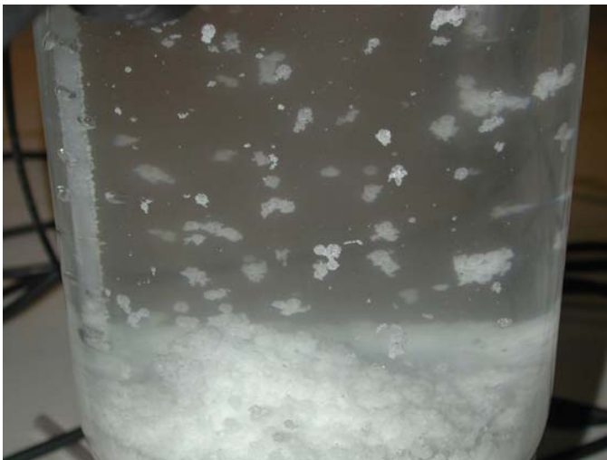
Figure 14 Sand aggregation with buoyant aggregates for a test with Inhibitor N and Oil 3. Test conditions: 10 %(w/w) NaCl, 60 °C, 0.8 bar CO 2 , pH 4.5, 10 % Oil 3.
