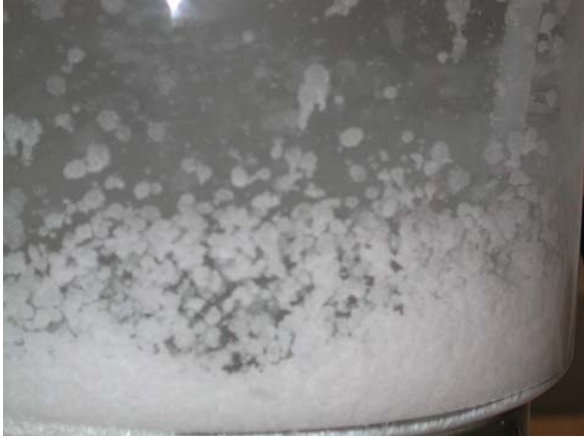
Figure 13 Sand aggregation with cake formation and sand sticking to walls for a test with Inhibitor M and Oil 3. Test conditions: 10 %(w/w) NaCl, 60 °C, 0.8 bar CO 2 , pH 4.5, 1 % Oil 3.
