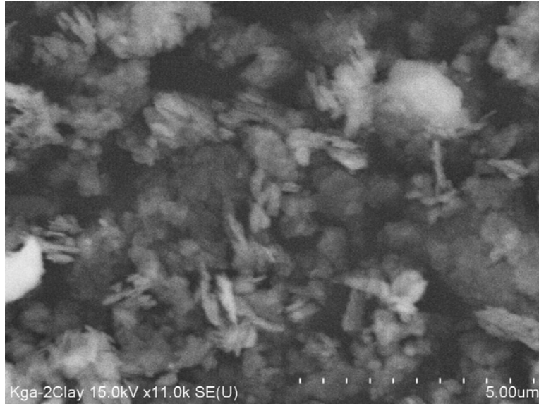
Figure 2 SEM image of KGa-2 kaolinite clay from Clay Mineral Society. 9 The clay flakes are 0.1-0.5 \mu\text{m} thick and 0.5-1 \mu\text{m} long.
