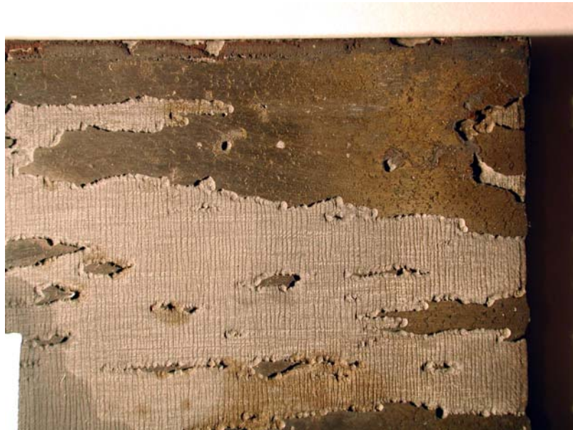
FIGURE 4 - Corrosion attack obtained in a test with a few ppb antimony, 0.2 MPa CO 2 partial pressure, pH 5. Two phase gas-water flow, 60 °C. The system was undersaturated with respect to FeCO 3 . Magnification about 2x.
