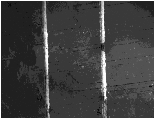
Fig. 5. The figure shows an image taken with the CCD-camera image of the hotspot described above (Fig. 4). The heat evolves at the precise location of a weak spot in the finger contact.
