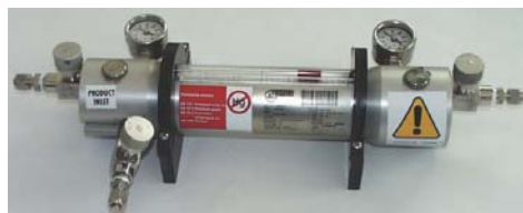
Pressurized gas tracer sampling cylinder with volume of 500 ml and typical pressure of 30-60 bar previously used for PFC-tracers and presently used for SF 4 and radiolabelled hydrocarbons
