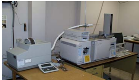
GC-MS with ATD for gas tracer analyses where CATS technology is applied
