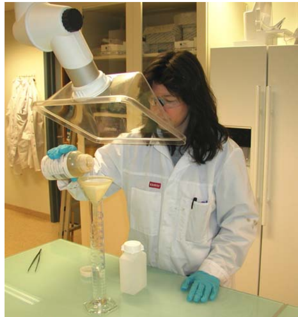
Filtration of water samples
